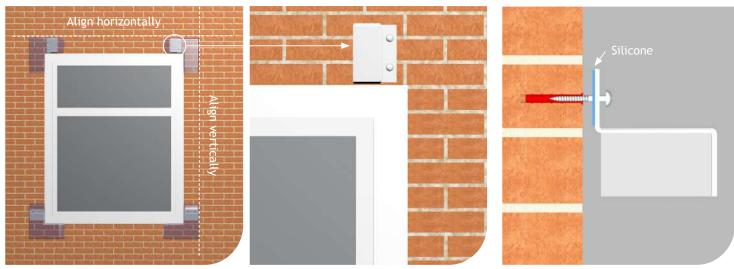
2. Position corners to accurately mark the position of the fixing bracket. It's important at this stage to align vertically and horizontally. (This ensures that the straight lengths in between corners will align properly).
