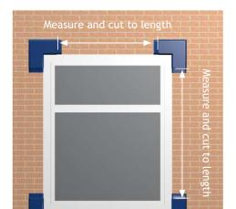
**5.** With all corners firmly in position, measure and cut the straight lengths to size.
