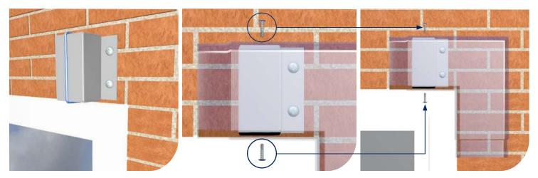
4. Apply a bead of silicone to the bracket. Fix the corners to bracket with appropriate aluminium fixings (use colour matched low profile self-tapping screws (see point 8)
