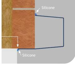
**9.** Seal the inside and outside edges by applying a finishing bead of silicone (colour matched or transparent).
