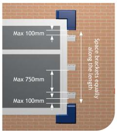
6. Fit the remaining brackets. Fit brackets at maximum 100mm from each corner and at maximum 750mm centres along the length.
