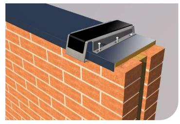
Position bracket with EPDM seal centrally over the wall. Maintain a minimum 10mm gap from the bracket inside return edge to the external wall surface finish (see Point 4 and also refer to Point 7). Brackets should be spaced at the correct centres according to the recommended number of brackets (please refer to Skyline Technical data for information).
