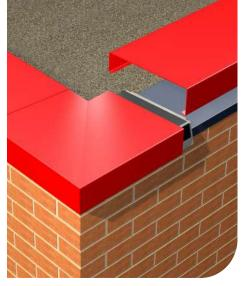
8. Start at a corner working to your next junction. The last section of coping can be cut down on site to accommodate any variant dimensions between corner, pier and stop ends. Use touch-up paint on cut edges. When cutting, make sure to use the correct metalwork tools to obtain a clean cut and dress any sharp burr edges.
