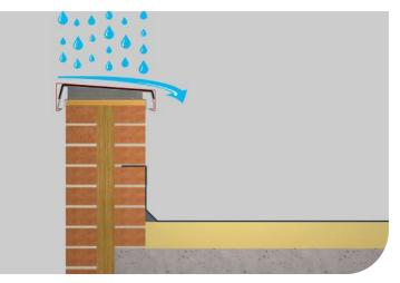
2. Skyline Sloped Coping is manufactured with an integral 20mm fall. Always install with the fall sloping towards the roof area. This ensures that rainwater run-off will be directed back onto the roof area.
