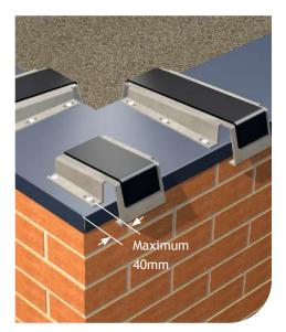
Always secure additional half brackets for corners and piers – the first fixing point with a maximum of 40mm from the external wall finish.
