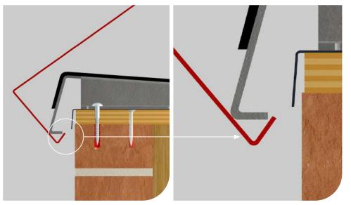
6. The coping simply pivots over the coping brackets and clips into position. First locate the front edge, and pivot over the bracket whilst slowly pressing the coping section into place to compress the EPDM seal on the brackets. Expect some resistance and apply consistent pressure and continue to press until it clips over the other edge of the bracket. The same method applies to Corners, T-Junctions and stopends.
