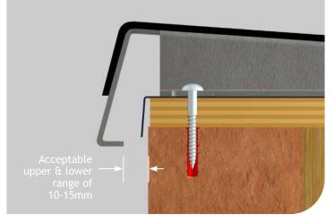
4. Secure coping bracket with high quality fixing (Minimum 50mm) appropriate for the substrate. The bracket has predrilled fixing holes which are provided as guidance only. Use the outermost fixing points to ensure maximum anchor point of the bracket to the wall. If fixings penetrate the masonry below, then ensure that the fixing is sufficiently back from the face to avoid damaging the masonry.
