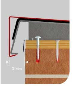
7. Ensure 31mm dimension is maintained from external wall surface finish to external face of coping. On deeper edged coping that exceeds the normal 85mm leg, it may be necessary to use a small selftapper on the coping return to secure it fully.
