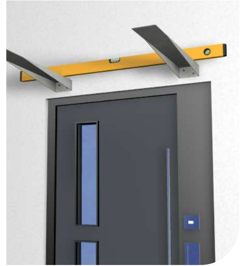
3. Level the wall bracket with a spirit level and check the position of the second wall bracket. Fit the second bracket into position. Double check level after fixing, and adjust or pack as required.
