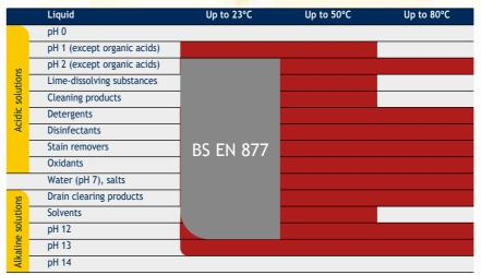
Conditions where interior coatings meet chemical resistance requirements of BS EN 877
