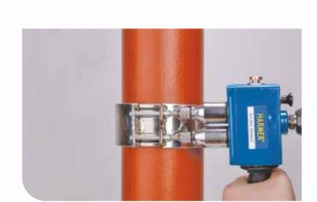
5. The Harmer Duomat fixing tool is recommended for securing Harmer Duo couplings. Bolts can be tightened simultaneously with precision.
