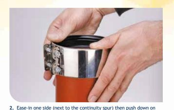
the opposite side of the coupling to fully seat, ensuring that the central inner register is abutted against the spigot end.
