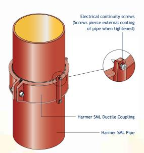
Harmer Ductile Coupling installation
