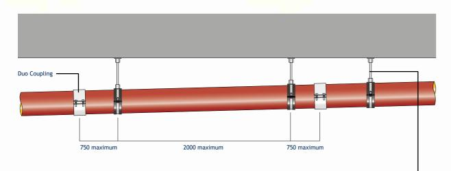
It is recommended that each pipe length in a horizontal pipe run should be supported by 2 brackets, not more than 2m apart. The length of pipe between a bracket and a coupling should not exceed 750mm.
