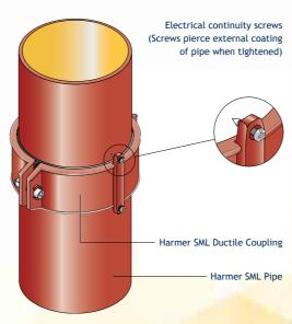
Harmer Ductile Coupling installation
