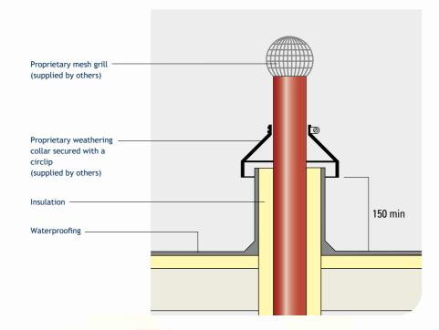
Standard specification guidelines for a 100mm diameter Harmer SML soil and waste system are provided below. NBS format specifications (R11 Above-Ground Foul Drainage Systems) are available for download on the Alumasc website.
