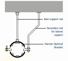
The requirement for pendular restraint may be removed if the pipework has branches entering at 45° or 90° which are supported by at least two hangers.
