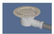
Connecting to 43mm  $(1^1/2^n)$  Polypropylene. Use 50mm to 43mm  $(1^1/2^n)$  proprietary solvent cement/compression reducer.
