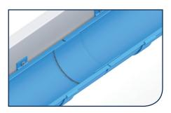
**Gutter Jointing** Joint sealing must not be carried out in wet weather or in temperatures below 5°C or above 40°C. Do not allow sealant applied to gutter joints to skin over or cure (>5 mins) before fitting unions or stop ends.
