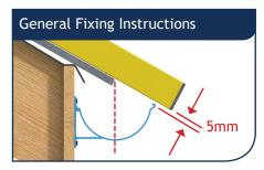
1 Using a straight edge, shim gutter brackets with 5mm clearance so that the last roof tile or slate will align with the midpoint of the gutter.
