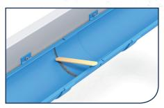
9) Tool-off displaced silicone sealant from the newly formed gutter joint. Allow to cure for 24 hours
