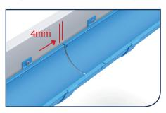
5) When joining gutter lengths, allow for a 4mm expansion gap.
