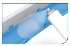
6) De-grease and clean each union and gutter length/ fitting to 50-100mm from the end.
