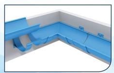
4) Offer angle pieces and outlets to the fascia. Lower gutter sections onto brackets leaving a 4mm expansion gap between gutter sections and allow enough clearance for the gutter joint before clipping gutter into brackets.
