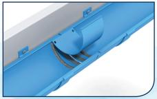
8) Place union centrally over prepared gutter joint and press firmly into the gutter until both edges of the union have engaged with gutter and union is secure. Excessive sealant will increase the force required to engage the union into the gutter.
