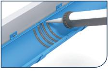
7) Apply two 4-6mm beads of Dow Corning 791 lowmodulus Type A silicone sealant to ends of gutter profile. Silicone sealant must be applied only to completely dry surfaces.
