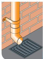
At ground level if the rainwater pipe does not connect directly to the gully, pipes can terminate with a shoe fitting for free discharge over the gully.
