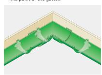
Plumb line outlets with gullies at ground level. Position angles, allowing an additional bracket adjacent to the joint with the gutter length.
