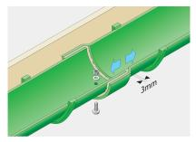
Insert the spigot end of the gutter allowing a 3mm expansion gap. Secure joint using aluminium M6 x 20mm nut, bolt and washer provided. (Bolt head preferably to underside).
