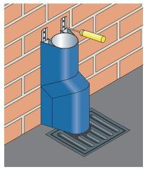
Commence installation by fitting fixing plates to the drain connector component and then fixing to the wall.
