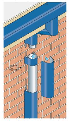
Build up and trim stack to within 300/400mm of underside of gutter and secure with fixing plates.
