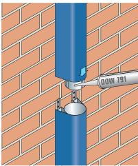
Pipe lengths are connected by sliding new pipe sections down over the fixing plates of the pipe below.
