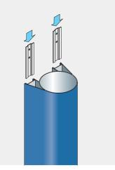
When joining pipe lengths tap two fixing plates per pipe connection into the pipe receiver rails using a block of wood to prevent damage.
