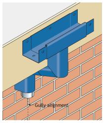
Guardian pipes are assembled from ground upwards.
