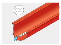
Pre-insert slide lock bars (1 per joint).
