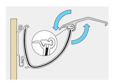
Reverse tool apply equal pressure around pivot point to complete lock bar positioning fully across joint. Take care not to dislodge gutter from fascia bracket.
