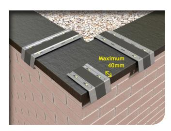
3. Secure brackets with minimum size No.12 x 50mm sized round head screws using the outer slots in the fixing straps at 1.5m maximum centres or as recommended based on wind uplift calculations or coping size. Additional screw fixings will be required on wider fixing straps. Maximum 40mm from fixing screw centre to external wall finishing surface.
