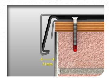
5. Locate the corner, and clip the coping edge angle under the bracket from the front whilst slowly pressing the coping section into place to compress the EPDM seal on the brackets. This also applies to a pier and stopends.
