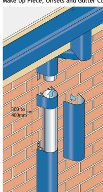
Build up and trim stack to within 300/400mm of underside of gutter and secure with fixing plates.
