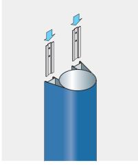
When joining pipe lengths tap two fixing plates per pipe connection into the pipe receiver rails using a block of wood to prevent damage.
