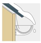
Fix brackets so as to position the gutter centrally and as close below the roof edge as possible, taking into consideration locality and roof slope finish. If there is a risk of sliding snow, adjust
