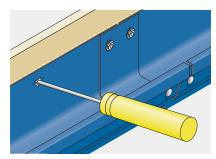
Tighten all fascia fixing screws and fit top straps if required otherwise screw back securely to the fascia using No12 x 38mm round head wood screws and washers provided.
