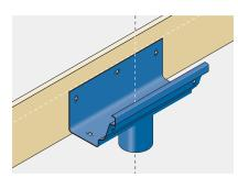
Plumb line outlet positions with gullies at ground level and mark fixing positions. Pilot 3.5mm diameter holes and loosely fit using No12 x 38mm round head wood screws and washers provided.
