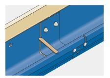
Tool off excess silicone and cone-off the exposed washers and nuts inside the gutter with a generous application of silicone sealant.
