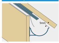
Using a straight edge or ruler, shim gutter brackets with 5mm clearance so that the last roof tile or slate will align with the mid point of the gutter.
