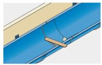
11. Tool-off displaced silicone sealant to the inside of the gutter joint. Tighten fixing bolts. Cone-off bolts and any other potential leakage points with sealant. Allow to cure for 24 hours.
