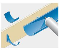
8. De-grease and clean each union and gutter length/fitting to a distance of 50 - 100mm from the end.
