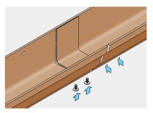
Secure the union to the gutter using the M6 x 20mm aluminium nuts, bolts and washers supplied. Pass bolt from outside in, and use washer and nut to secure finger-tight.
