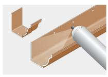
7. De-grease and clean each union and gutter length/fitting to a distance of 50mm - 100mm from the end.
