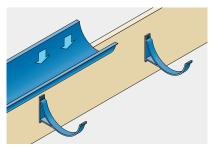
6. Clip gutter sections into brackets.
