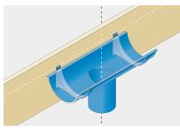
4. Plumb line outlet positions with gullies at ground level.
