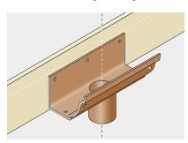
4. Plumb line outlet positions with gullies at ground level
