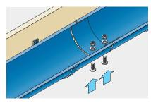
Secure the union to the gutter using the M6 x 12mm aluminium nuts, bolts and washers supplied. Pass bolt from outside in, and use washer and nut to secure finger-tight.
