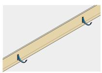
Use a string or laser to establish a true line and level of the gutter. Prepare to use packing pieces under brackets where there are depressions.
